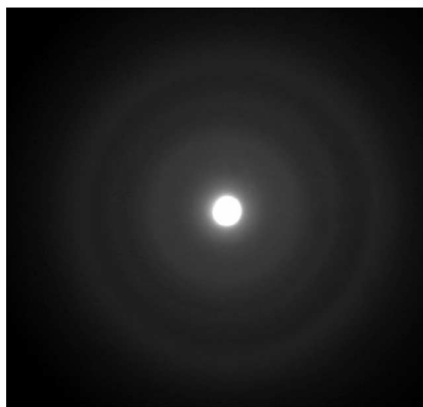
Fig. 5. SAED pattern measured from \text{RuO}_{1.0}(\text{OH})_{1.0} \cdot 0.60\text{H}_2\text{O} that was annealed at 116^\circ\text{C} and then reacted with methanol.
